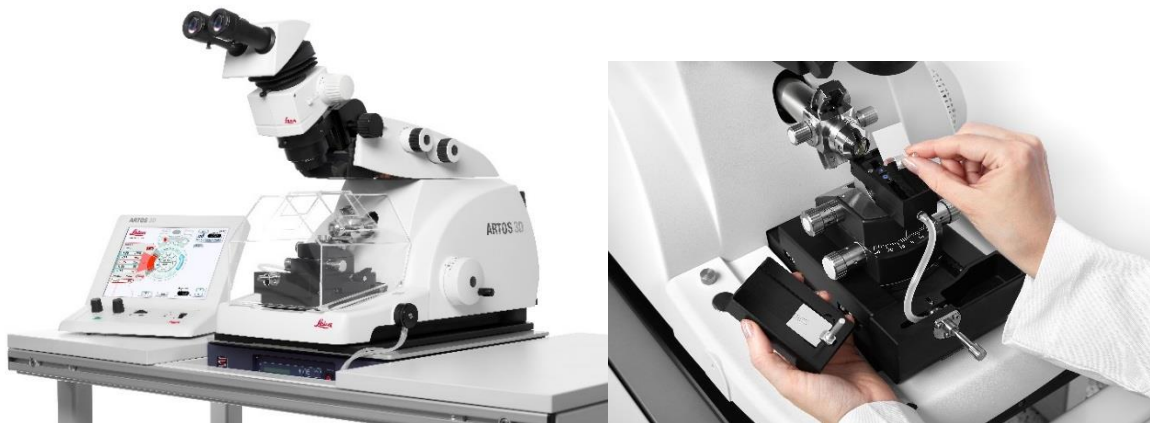
Figure 1: ARTOS 3D (Left) and its collection method of serial sections (Right).
