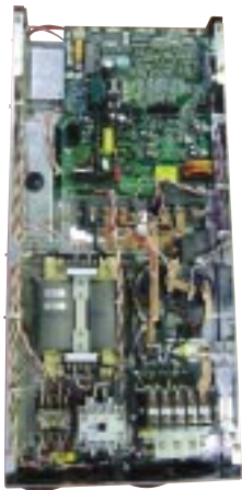
Battery Controller for Elevator
