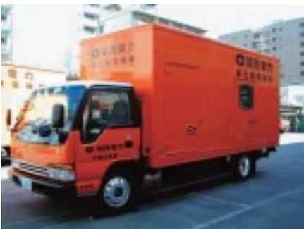
*500kW Diesel Engine High-Voltage Generating System*
