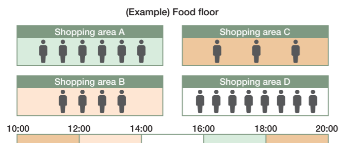
AI analyzes congestion and time of day, and adjusts the air conditioning environment to suit each sales floor
