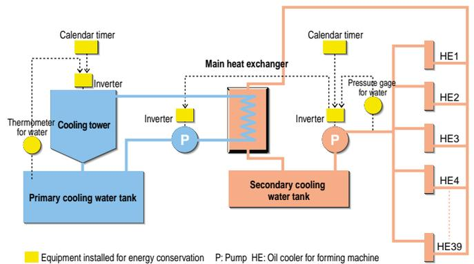
■ Equipment installed for energy conservation P: Pump HE: Oil cooler for forming machine
