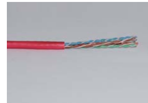
1. Stripping off 1 inch (2.5cm) of jacket from end.
