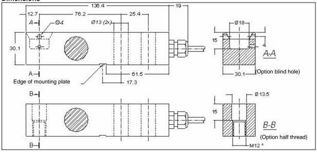
All dimensions in mm. Dimensions and specifications are subject to change without notice. Mounting bolts for 200 lb to 2500 lb: M12 8.8 / torque 90 Nm; for 5000 lb: M12 10.9 / torque 120 Nm. Torque values assume oiled threads.
