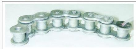
Photo of CR-Chain after Salt Spray Test of 1200hrs
