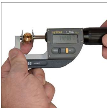
Part measurement with a S_Mike PRO Disk
