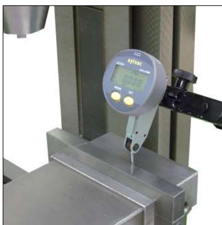
Checking the alignment on milling machine.
