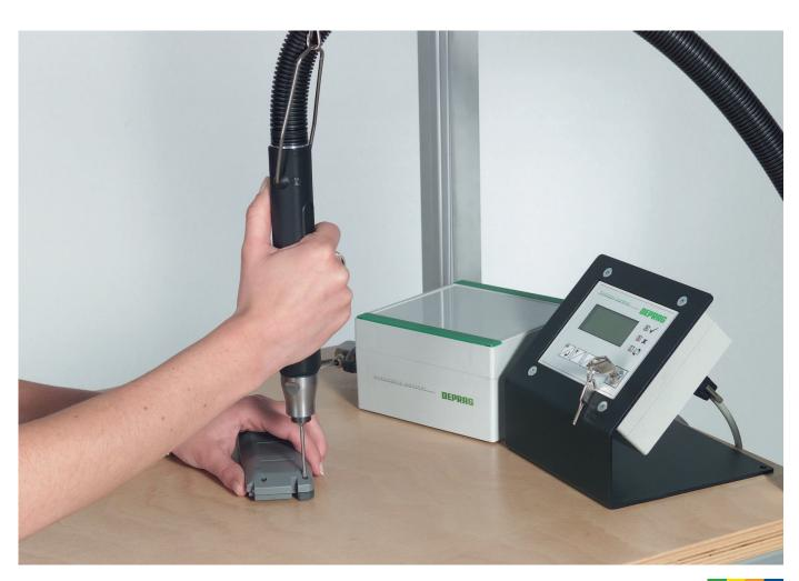
With activation of the driver, the airflow is released through the newly designed and improved controller fc10 in connection with the pneumatic controller pc10. When the preset torque is reached, the driver shuts off using the highly accurate shut-off clutch of the screwdriver series MINIMAT. The integrated function-recognition reports the completion of the screwdriving cycle to the controller fc10.
