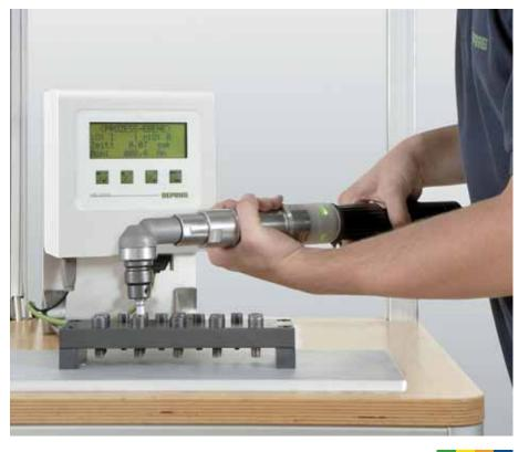
The QC Screwdriver of the MINIMAT-series is a pneumatic tool with control functions for a 100 % process quality of assemblies. In addition, the manual QC Screwdriver is able to register the reached torque values, achieved with the highly precise shut-off clutch. Based on a strain gauge torque transducer the values can be displayed and stored via the respectively connected measuring electronic of the new controller family, type ME 1000 QC.
