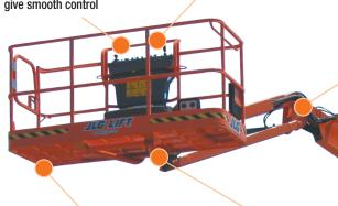
Jib boom and basket rotate allow additional functionality and access to hard to reach positions
