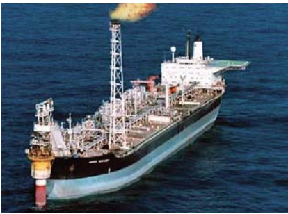
Floating, production, storage and offloading (FPSO) facility operating in East Timor
