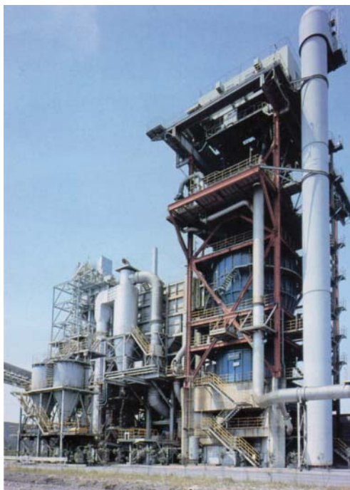
Coke dry quenching equipment delivered to POSCO of the Republic of Korea in conjunction with Nippon Steel Corporation and POSCO Engineering & Construction Co., Ltd.
