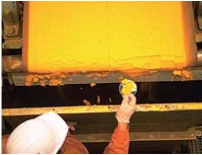
A view of "yellowcake," so called because of the yellow color of uranium just after production from uranium ore. With great energy potential, it is processed into fuel for nuclear power generation, which accounts for more than 30% of total electric power in Japan. [Photo: COGEMA]
