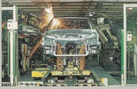
Welding assembly process for car bodies
