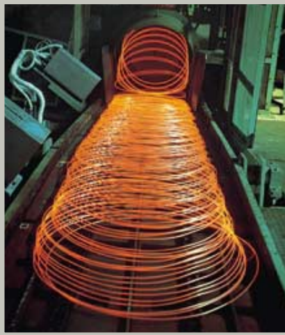
Wire rod coming off a rolling line
