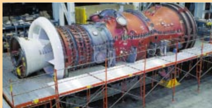
Gas turbine for Combined Cycle Power Plant
