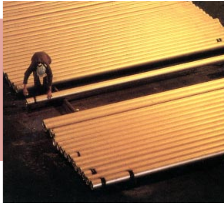
Ultrasound inspection of steel pipe
