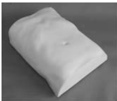
Figure 3. Overall view of the abdominal model featuring an adult male's torso from chest to lower umbilical region, coated in silicon
