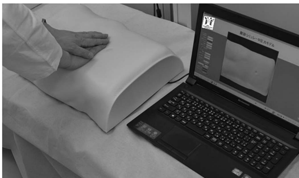
Figure 3. View of the complete abdominal palpation monitoring system including abdominal model and PC.
