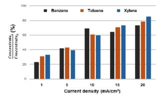
Fig.l: High concentration of VOCs removal efficiency according to current density at 2.8 cm electrode gap after 40 mins.
