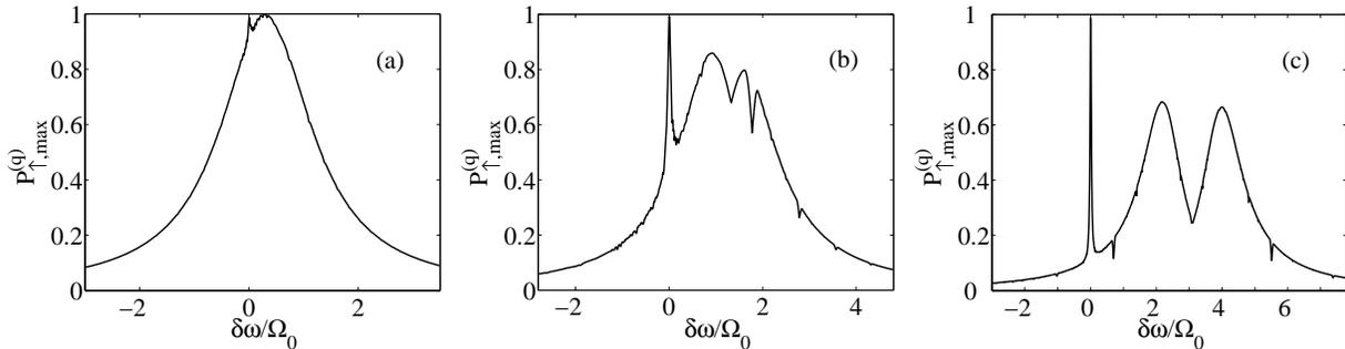
Figure 2: Maximum qubit excitation probability  $P_{\uparrow, \text{max}}^{(q)}$  between  $t = 0$  and  $t = 20\pi/\Omega_0$  for  $\lambda/\Omega_0 = 0.5$  (a), 2 (b) and 5 (c).  $\theta_q = \pi/4$ , and  $\theta_{\text{TLS}} = \pi/6$ .
