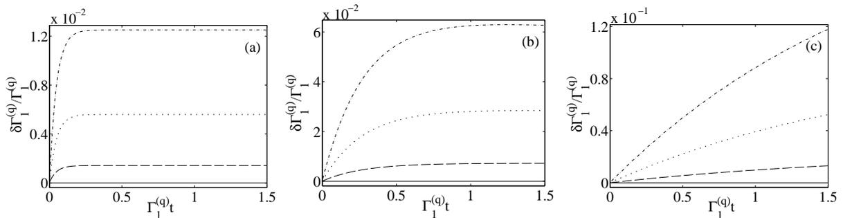
Figure 1: Relative corrections to qubit relaxation rate as a function of scaled time in the case of (a) strongly, (b) moderately and (c) weakly dissipative TLS. The ratio  $\Gamma_1^{(\text{TLS})}/\Gamma_1^{(q)}$  is 10 in (a), 1.5 in (b) and 0.1 in (c). The solid, dashed, dotted and dash-dotted lines correspond to  $\lambda/\Gamma_1^{(q)} = 0, 0.3, 0.6$  and  $0.9$ , respectively.  $\theta_q = \pi/3$  and  $\theta_{\text{TLS}} = 3\pi/8$ .
